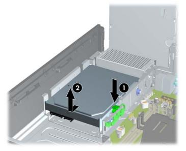
8. To install a hard drive, you must transfer the silver and blue isolation mounting guide screws from the old hard drive to the new hard drive.
